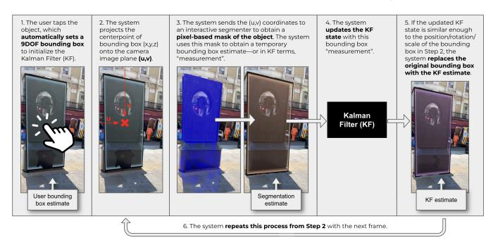
Figure 7: A visualization of the Landmark Tracker algorithm, which we developed to reduce drift of the *Object Transform* in the full-study apps.
