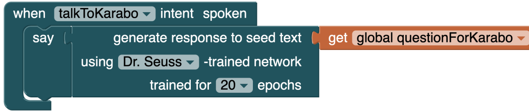
Figure 2-8: The endpoint event for the talkToKarabo intent. These blocks cause Alexa to respond with a uniquely generated sentence that may sound similar to a sentence Dr. Seuss came up with.
